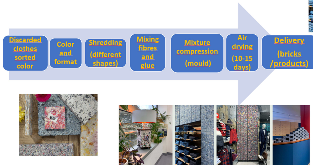
Fig. no. 27 Mechanical recycling by FabBRICK 80
